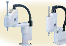
Synchronous control of two SCARA robots
