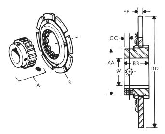
The Ajusto-gap® feature is used to give a positive release of the armature plate while maintaining a constant air gap throughout the wear life of the unit.
