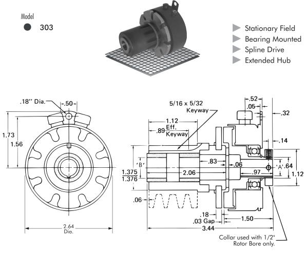
Customer to supply set collar/retaining device to maintain axial position of extended hub on shaft.
