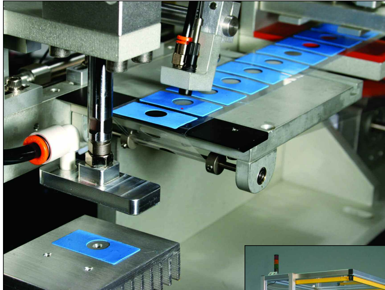
The COBRA Placement System automatically and accurately places components to \pm .005 ".
