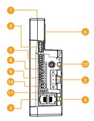
1 Serial Port 2 Power Supply 3 Ethernet Port #1 4 Ethernet Port #0 5 USB Host
