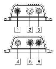
1 Power supply, serial port 2 USB port 3 CAN port 4 CAN port 5 Ethernet port 1 (10/100 Mb) 6 Ethernet port 2 (10/100 Mb)
