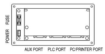
The product is compatible with all standard TCM and SCM modules. To access the slot for the modules, remove the rear cover of the product
