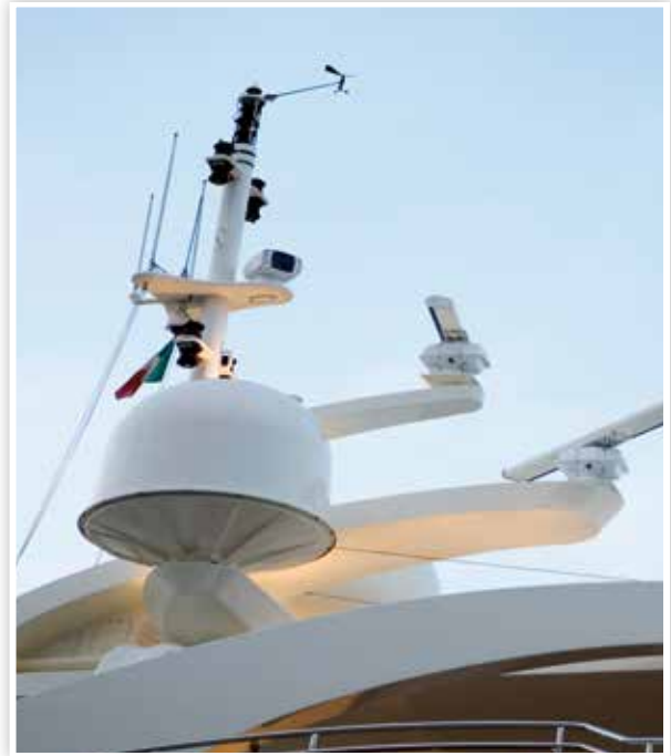
A highly reliable brushless DC motor keeps this satellite antenna on track in a harsh and demanding marine environment.
