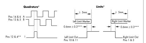
\*Output signals are IEEE 422 compliant, 3.3V differential logic.
