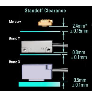
\* Dimensions shown illustrate encoder system standoff clearance; see Mercury Encoder Interface Drawings for correct design reference surfaces.
