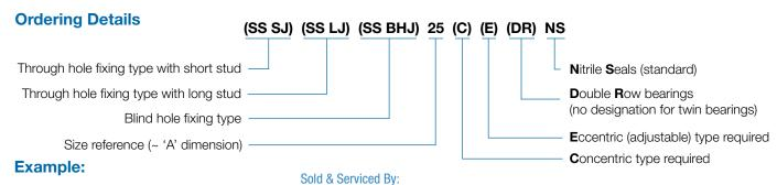
2 x SS SJ 34 C NS Stainless steel short stud size 1 concentric bearing assemblies with twin bearings and standard nitrile seals 2 x SS SJ 34 E NS Stainless steel short stud size 34 eccentric bearing assemblies with twin bearings and standard nitrile seals 10 Free Phone (877) SERVU98
