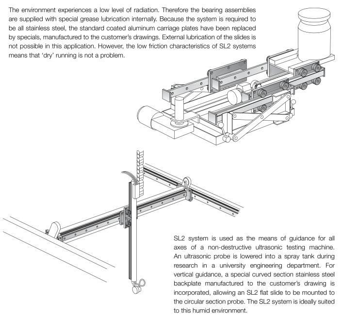
The use of twin type bearing assemblies offers extra compliance to compensate for slight deviations of the opposing slides on the horizontal axis. Lubricators give increased system life while retaining low friction. The zero play which is characteristic of the SL2 system ensures rigidity at the probe end, despite the large overhang in this application.
