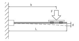
In the equations (1) and (2) above, L, k and d are the dimensions shown in the relevant diagrams (in mm) and F is the load applied in Newtons. The term Rc is a constant relating to the stiffness of the flange clamp, and El is the product of the material's Young's modulus and the section moment of inertia, which is a constant relating to the stiffness of the slide section in the orientation of the application\*. These constants are given for the various systems in the table below.
