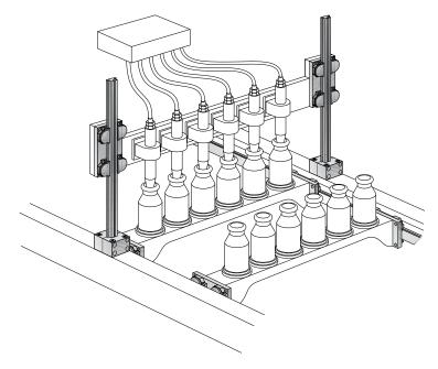
SL2 system is used as the vertical guidance in a food industry application to move a diverting conveyor between two further conveyors alternately. High speed and high duty operation driven by a crank arm.
