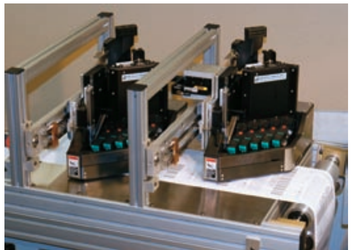
This variable media printer utilizes a horizontally mounted un-driven LoPro to manually position print heads and a pneumatically driven UtiliTrak to vertically position UV curing heads.
