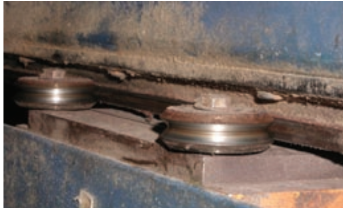
Guide wheel technology provides unmatched reliability in harsh environments. The wheel's inner vee diameter travels at a slower rate than the outer vee diameter, resulting in a velocity gradient that sweeps aside any debris that has settled on the track.
