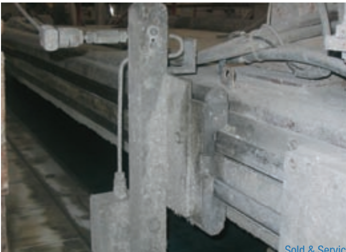
Designed for extreme environments and caked in cement dust, this size 4, belt-driven LoPro reliably drives a water jet cross cutter on a cement fiberboard plank siding line.
