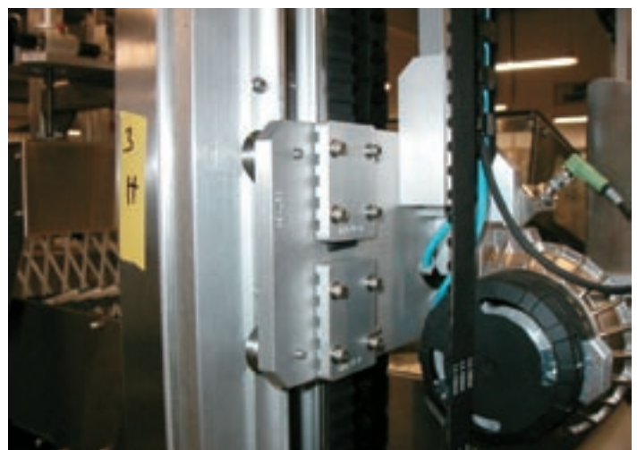
DualVee wheels and pre-mounted track plates provide an effective and compact method to raise, lower and guide a bucket full of products from one conveyor line to another for this pharmaceutical, cosmetic and personal care packaging machine.
