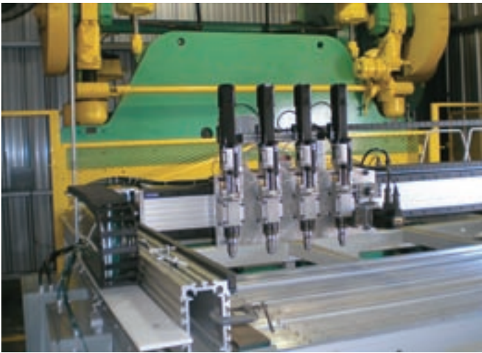
HepcoMotion HDS Heavy Duty Slide system provides rigidity and accuracy for an automated multi-head drilling machine. HDS handles the high load requirements and every day pounding with ease.
