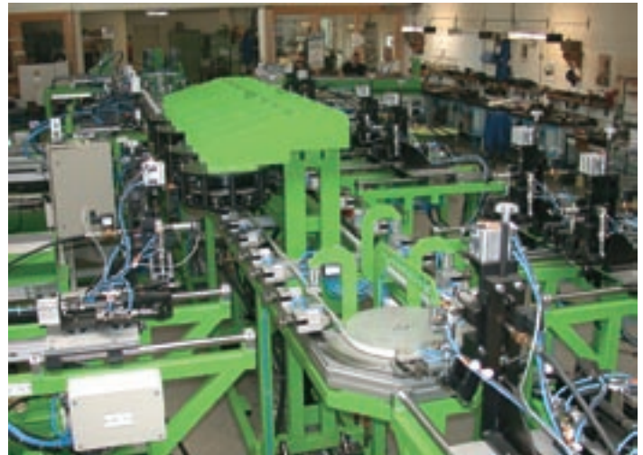
This handling & assembly system uses HepcoMotion DTS and PRT to cut, sort and transport washing machine hoses to an assembly station.
