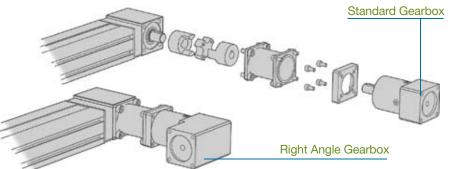
The example shown incorporates an AC inverter motor. This high performance system can deliver a linear force of 145N and speeds over 5m/s. Other motor combinations are available. Bishop-Wisecarver will supply fitted gearboxes with ratios from 3:1 to 512:1 complete with input flange to suit your motor.
