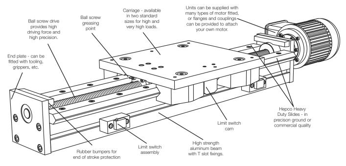
Hepco HDCS units can be supplied with many useful options including bellows covers, motors, couplings, flanges, T nuts, brackets etc. They can be used in multi-axis systems, which can be built by the customer or supplied complete by Bishop-Wisecarver.
