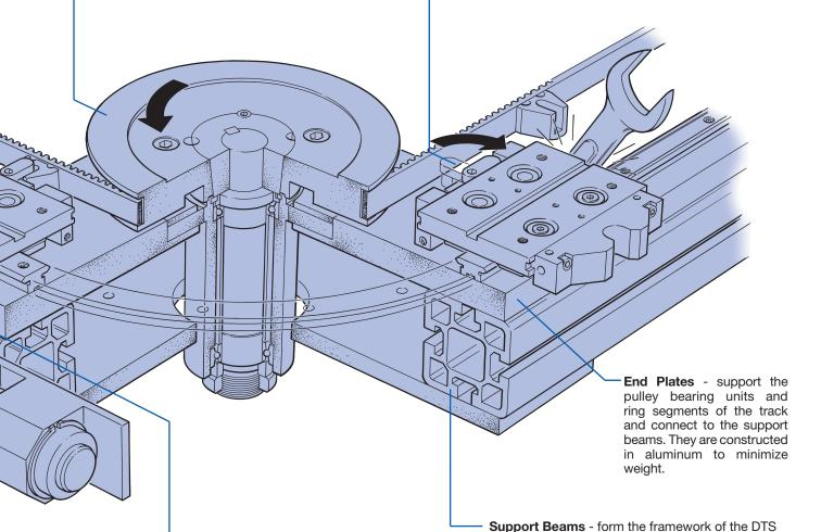
Sensor Mounting Brackets (optional) - can be positioned anywhere along a straight section and are available from Bishop-Wisecarver to suit M8 threaded proximity switches (not supplied).
