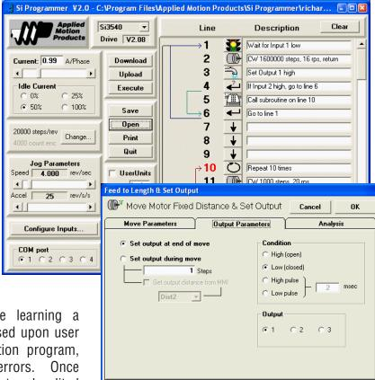
in  $Si^{TM}$  mode, the user can address their multi-axis applications with either the  $SiNet^{TM}$  Hub or  $SiNet^{TM}$  Hub 444, up to 8 drives can be connected to a host's serial port through one Hub.
