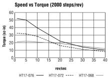
Speed vs Torque (2000 steps/rev)
