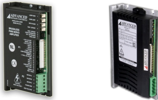
Figure 3 Existing brushless analog drive and new brushless AxCent drive
