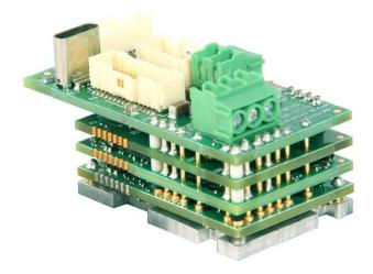
The **FM060-5-EM** is a single-axis servo drive and integration board assembly for a FE060-5-EM FlexPro<sup>™</sup> series servo drive with IMPACT<sup>™</sup> architecture. Connections to the controller, motor, power, and feedback are simplified through the standard connectors featured on the board.
