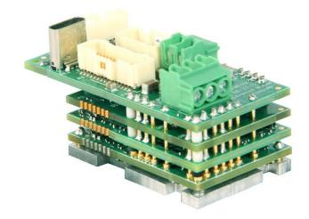
The **FM060-10-EM** is a single-axis servo drive and integration board assembly for a FE060-10-EM FlexPro<sup>™</sup> series servo drive with IMPACT<sup>™</sup> architecture. Connections to the controller, motor, power, and feedback are simplified through the standard connectors featured on the board.
