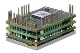
The **FE060-60C-EM** is a FlexPro® series servo drive with IMPACT™ architecture.
