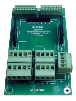
**DESCRIPTION:** The MC2XZQD mounting card is designed to host up to two Z Series servo amplifiers. These two amplifiers are installed in a stacked configuration to keep the footprint small while offering convenient pluggable screw terminals for easy interface connections. An amplifier mounting kit is included to secure the two Z Series amplifiers onto the mounting card.
