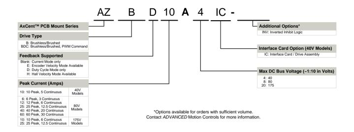
ADVANCED Motion Controls servo drives are available in many configurations. Note that not all possible part number combinations are offered as standard drives. All models listed in the selection tables of the website are readily available, standard product offerings.
