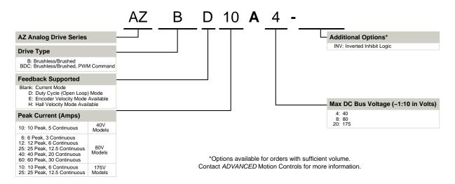
ADVANCED Motion Controls AZ series of servo drives are available in many configurations. Note that not all possible part number combinations are offered as standard drives. All models listed in the selection tables of the website are readily available, standard product offerings.
