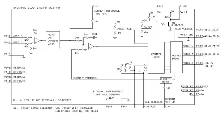
JE2- PHASING: 120 DEGREE WHEN INSTALLED, 60 DEGREE WHEN NOT INSTALLED
