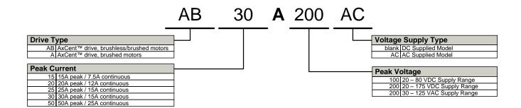
ADVANCED Motion Controls analog series of servo drives are available in many configurations. Note that not all possible part number combinations are offered as standard drives. All models listed in the selection tables of the website are readily available, standard product offerings.
