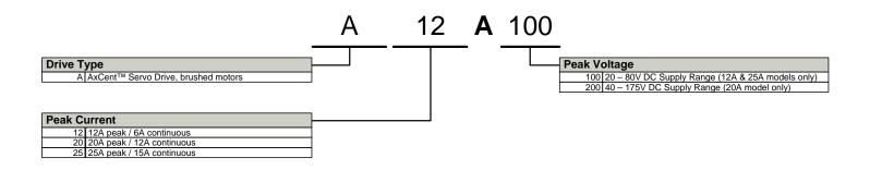
ADVANCED Motion Controls' AxCent<sup>™</sup> series of servo drives are available in many configurations. Note that not all possible part number combinations are offered as standard drives. All models listed in the selection tables of the website are readily available, standard product offerings.
