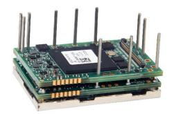
The **FXE060-5-CM** is a FlexPro<sup>®</sup> series Extended Environment servo drive with IMPACT™ architecture.
