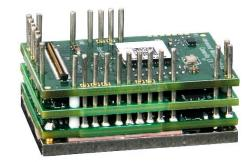
The **FXE060-10-EM** is a FlexPro<sup>®</sup> series Extended Environment servo drive with IMPACT<sup>TM</sup> architecture.
