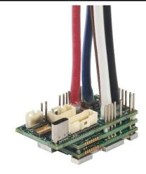
The **FM060-60C-CM** is a single-axis servo drive and integration board assembly for a FE060-60C-CM FlexPro® series servo drive with IMPACT<sup>TM</sup> architecture. Connections to the controller, motor, power, and feedback are simplified through the standard connectors featured on the board.
