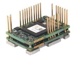
The **FE060-10-CM** is a FlexPro<sup>®</sup> series servo drive with IMPACT<sup>TM</sup> architecture.
