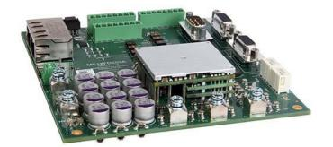
The **FD100-50-EM** is a servo drive and development board assembly for a FE100-50-EM FlexPro<sup>®</sup> series servo drive with IMPACT<sup>TM</sup> architecture. Connections to the controller, motor, power, and feedback are simplified through the standard connectors featured on the board. The **FD100-50-EM** is ideal for prototyping and can be used in production and industrial environments as well.
