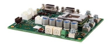
The **FD060-25-RM** is a servo drive and development board assembly for a FE060-25-RM FlexPro<sup>®</sup> series servo drive with IMPACT<sup>TM</sup> architecture. Connections to the controller, motor, power, and feedback are simplified through the standard connectors featured on the board. The **FD060-25-RM** is ideal for prototyping and can be used in production and industrial environments as well.
