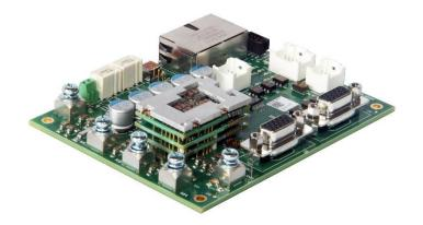
The **FD060-25-EM** is a servo drive and development board assembly for a FE060-25-EM FlexPro<sup>®</sup> series servo drive with IMPACT<sup>TM</sup> architecture. Connections to the controller, motor, power, and feedback are simplified through the standard connectors featured on the board. The **FD060-25-EM** is ideal for prototyping and can be used in production and industrial environments as well.
