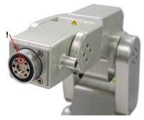
(a) The robot's flange at  $\theta_6 = 0^{\circ}$
