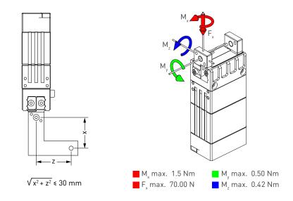
Figure 3: Maximum permissible finger dimensions and finger loads
