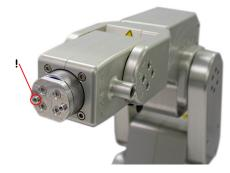
(b) The adaptor attached in the correct orientation
