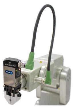
Figure 6: The MEGP 25E completely installed and homed
