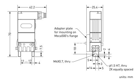
Figure 2: Dimensions of the MEGP 25E gripper
