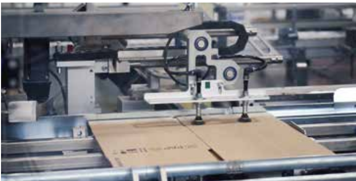
Stacking height measurement of cardboard
