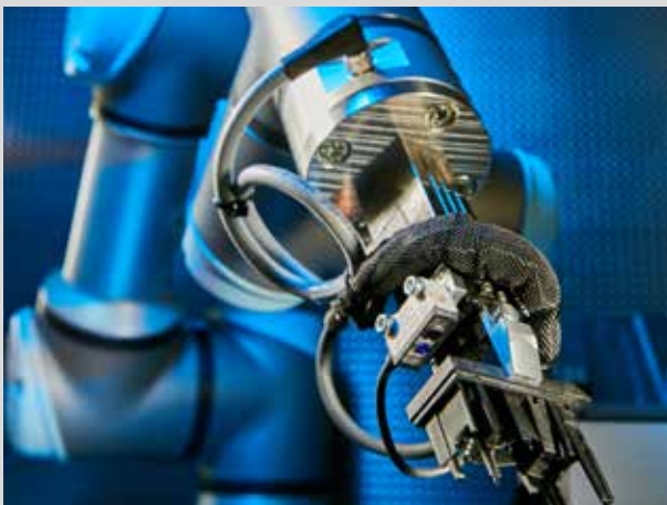
Distance measurement in robotics applications directly from the gripper
