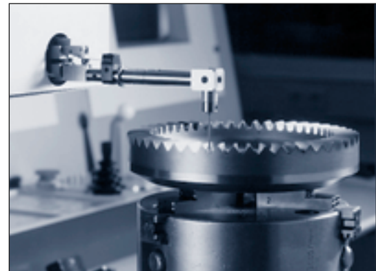
Computerized mapping of gear tooth profile
