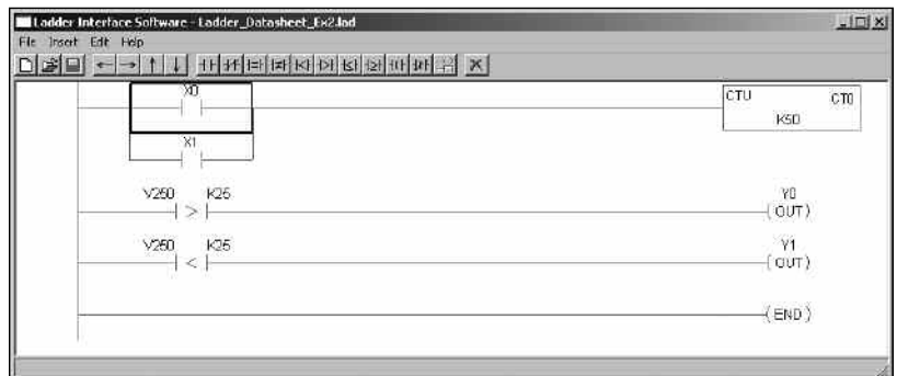
Up-Counter (CTU) and comparative logic example
