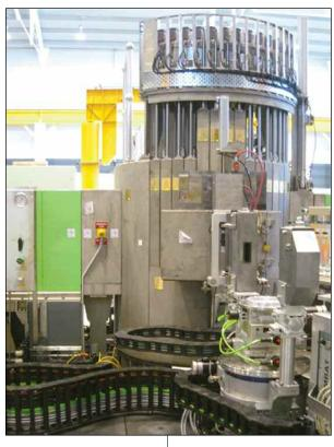
42 eight-axis Galil controllers help maneuver eight neutron beam instruments for scientific research.
