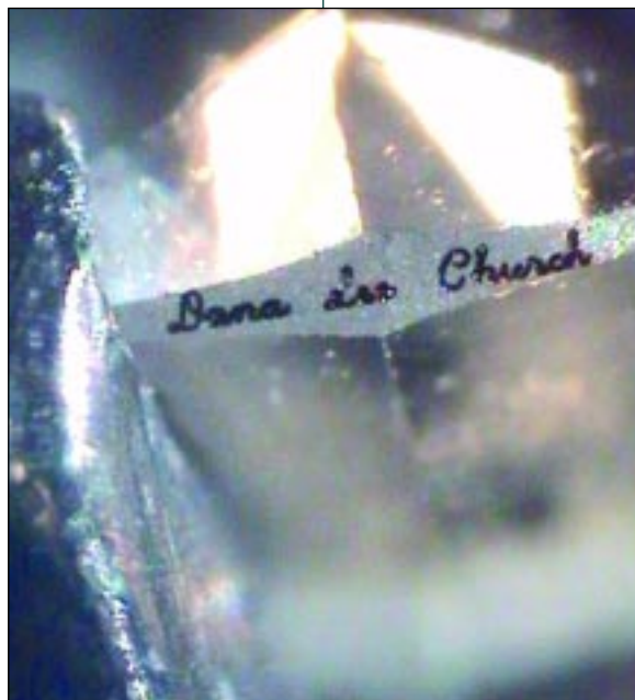
The PhotoScribe/TeoSys laser system engraves precisely on a diamond.
