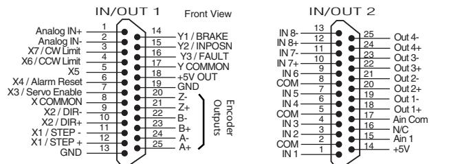
Note - this connector is standard on S version and only on S and Q versions with expanded I/O.
