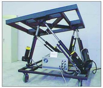
which are calculations that translate the X, Y, Z, Yaw, Pitch and Roll data into target positions—for each individual axis.
